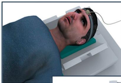
MoTrak Head Band with Motion Sensor
